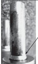
THIS CLUTCH HUB DRIVE PIN SHOWS EVIDENCE IT HAS BOTTOMED OUT ON THE DAMPER BUSHING. THE WEAR MARKS SHOULD NOT EXTEND TO THE BEVEL AT THE BASE OF THE PIN AS SHOWN HERE.
